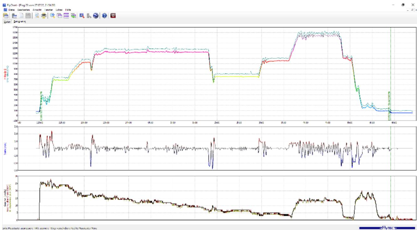
Complete documentation of the 8-hour course in the Flytec 6040: Note the stable altitude accuracy of 6-8 m standard deviation over hours, which can never be achieved by hand! The intermittent variations resulted from the bottle change and the subsequent manual burner tests. This allows the burning time of the individual cylinders to be easily assigned and verified.
